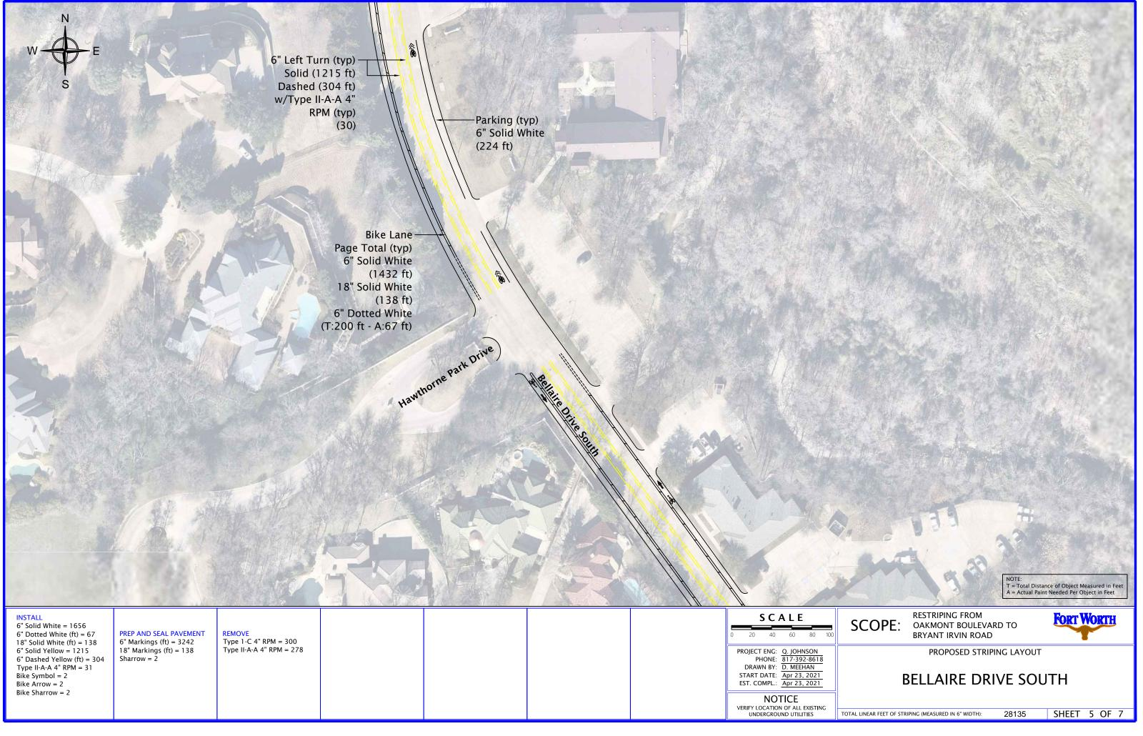
6" Left Turn (typ) Solid (1412 ft) Dashed (353 ft) w/Type II-A-A 4" RPM (typ) (35)
