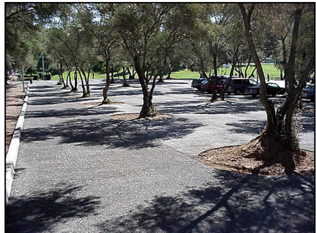
Trees planted in parking lots, together with pervious surfaces such as permeable concrete, improve environmental quality and help reduce stormwater runoff.
