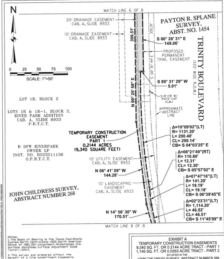
1. The Bosis of Bearing is the Texas Coordinate System, North Central Zone 4202, North American Datum of 1983, 2011 adjustment. All distances are surface distances. Surface Adjustment Scale Factor: 1.00012.
