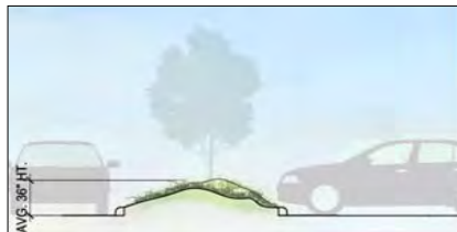
Section: Earthen-berm height requirements
