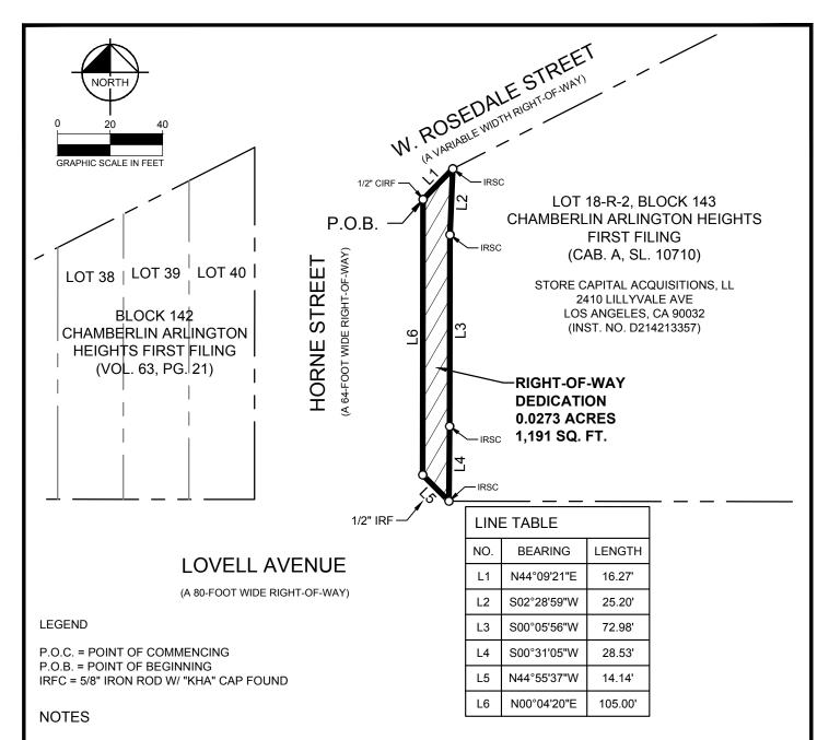
Bearing system based on the Texas Coordinate System of 1983(2011 adjustment), North Central Zone (4202). A metes & bounds description of even survey date herewith accompanies this survey plat.
