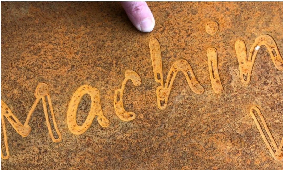
Fabrication sample: text on each of the four (4) 6' weathering steel panels to be incorporated Engraving 1/16" (example above) Engraving 3/16" Cut Out
