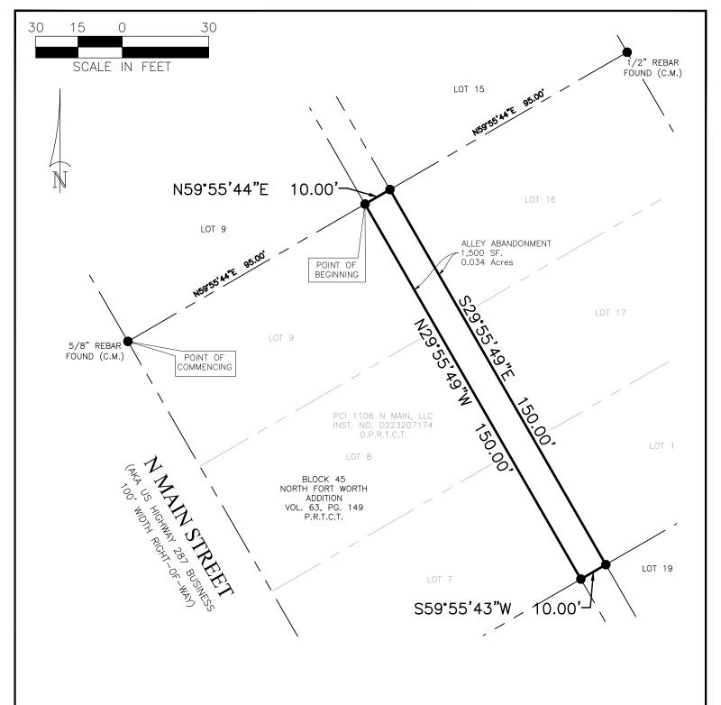
The Basis of Bearings is from the Texas State Plane Coordinate System, NAD83, North Central Zone as derived from GPS observations using the Allterra RTK Network and adjusted to surface using a surface scale factor of 1.00012.
