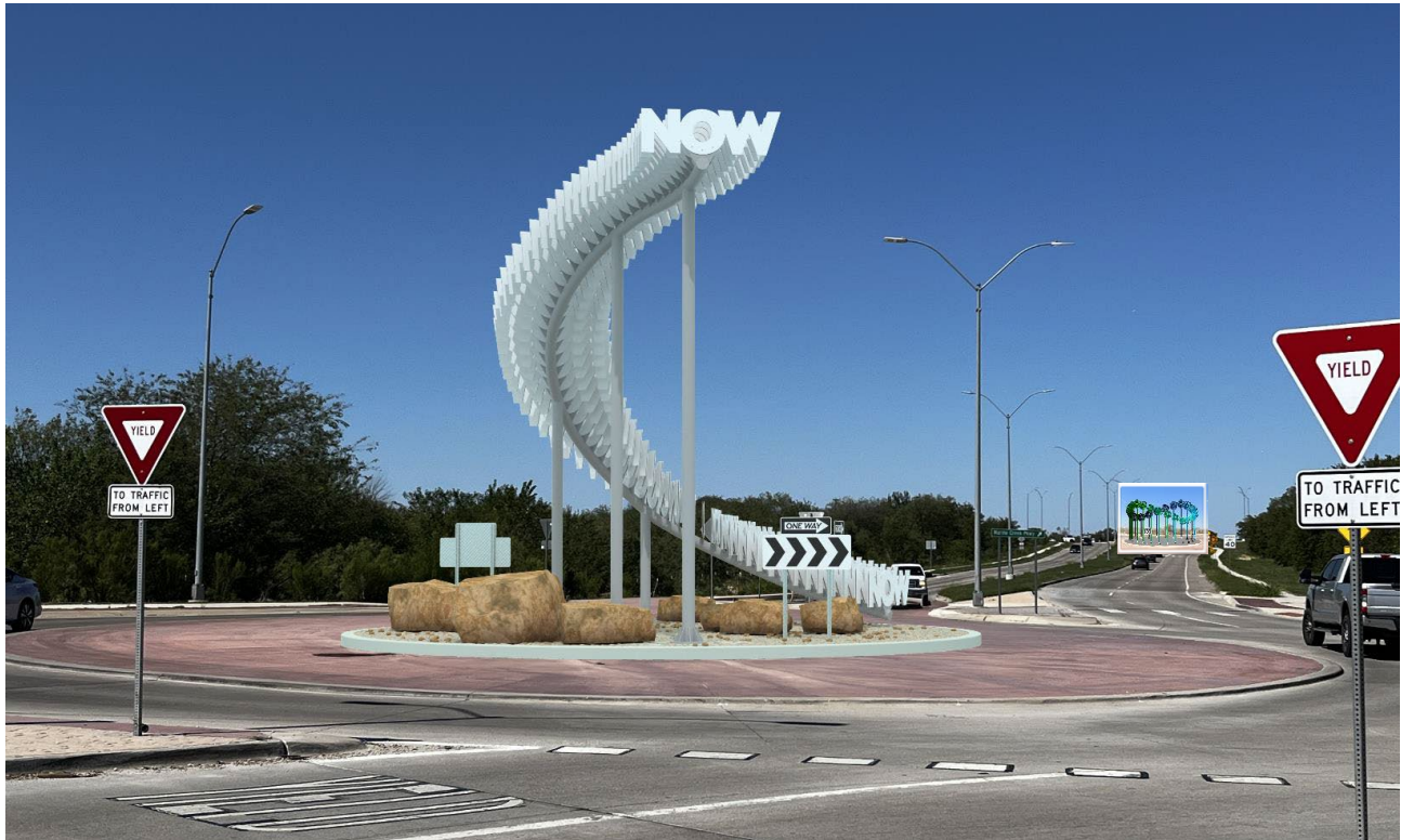
Final Design Rendering (Northbound View) 28 ft., 10 in. (h) x 35 ft., 9 in. (w) x 25 ft., 2 in. (d) Painted aluminum "NOWs" with steel support structure
