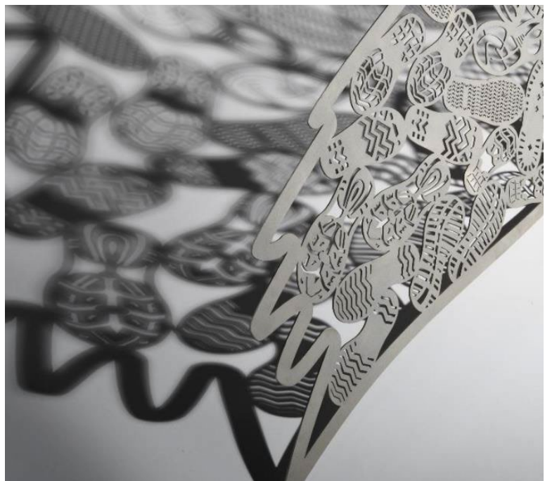
Laser-Cut Stainless Steel Wing Mockup with Sample Shoe Treads (10 total)
