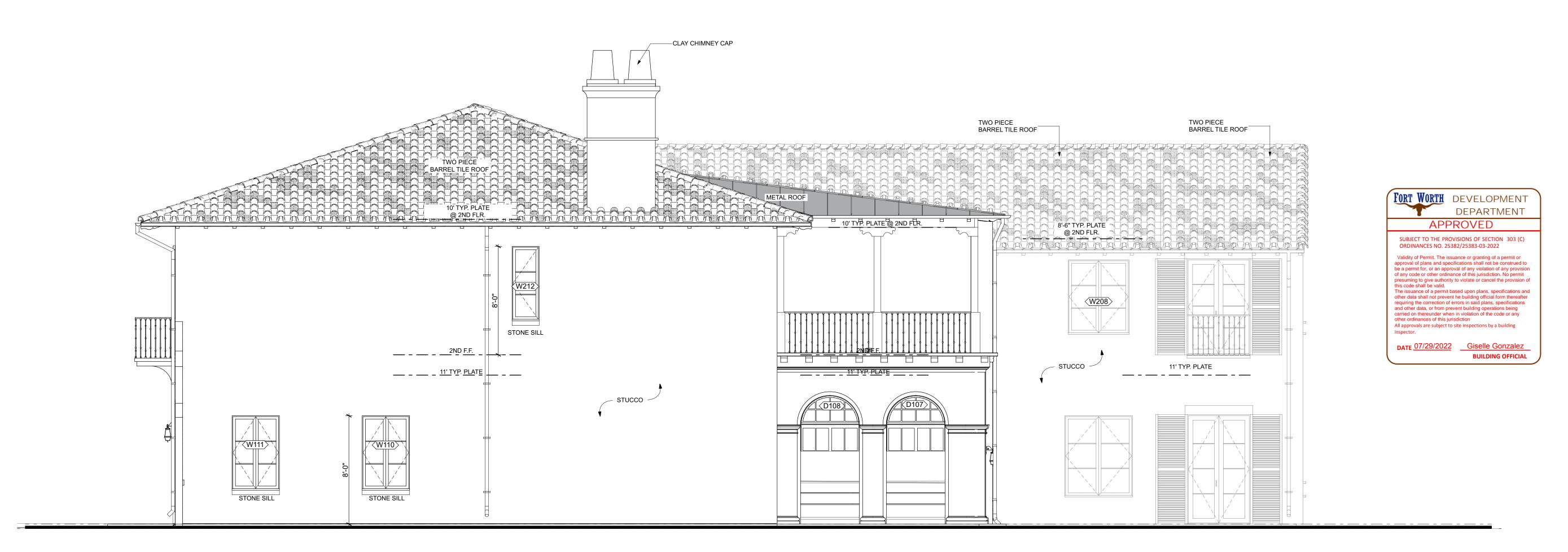
TWO PIECE BARREL TILE ROOF TWO PIECE BARREL TILE ROOF
