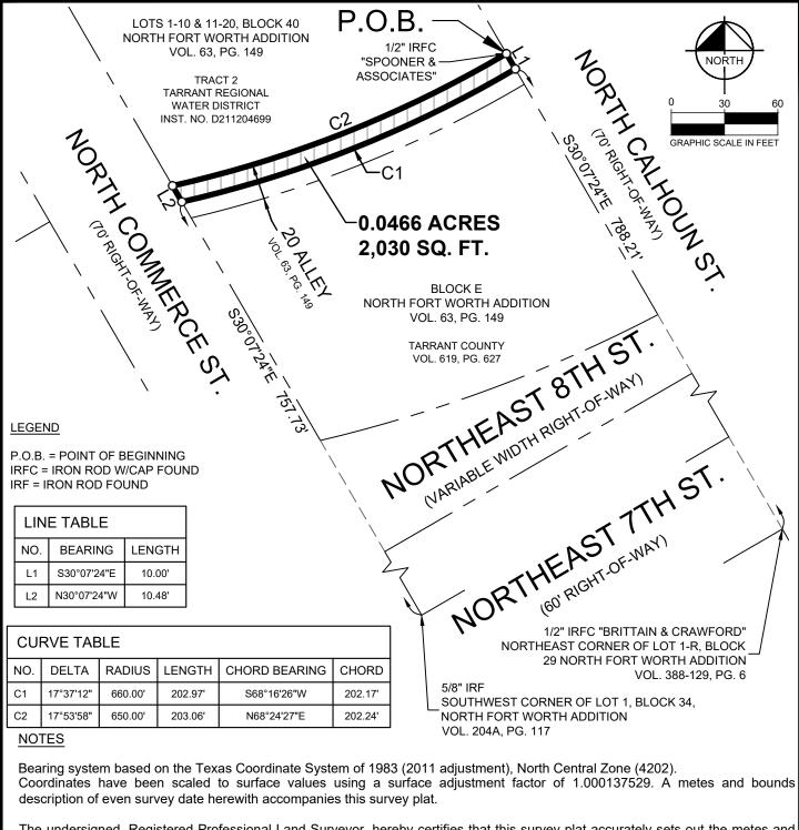
The undersigned, Registered Professional Land Surveyor, hereby certifies that this survey plat accurately sets out the metes and bounds of the abandonment tract. **RIGHT-OF-WAY ABANDONMENT**
