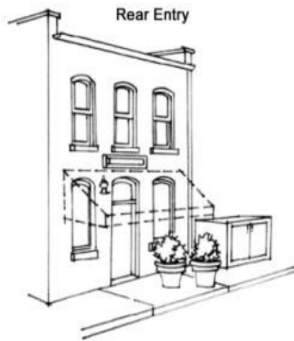
Example of a rear building elevation sign
