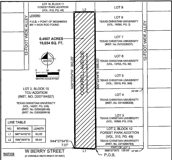
Bearing system based on the Texas Coordinate System of 1983 (2011 adjustment), North Central Zone (4202). A metes and bounds description of even survey date herewith accompanies this survey plat. Corners shown hereon are 5/8-inch iron rods with "KHA" caps set unless otherwise noted.
